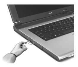
When the power is off, you can eject the drive tray using the emergency eject hole. See page 62.
