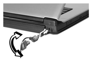
Wrap a computer security lock cable around an immovable object such as a table or handle of a locked drawer. Insert the lock into the notch and turn the key to secure the lock. Some keyless models are also available.
