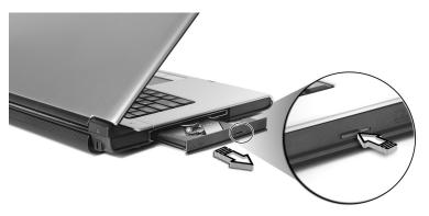
When the power is off, you can eject the drive tray using the emergency eject hole.
