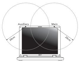
**Note**: Acer Wireless Mini PCI Adapter implements a transmission diversity function. The function does not emit radio frequencies simultaneously from both antennas. One of the antennas is selected automatically or manually (by users) to ensure good-quality radiocommunication.
