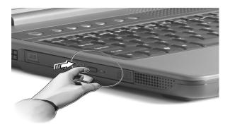
When the power is off, you can eject the drive tray using the emergency eject hole. See page 44.
