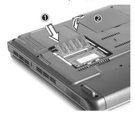
4 Replace the memory cover and secure it with the screw.
