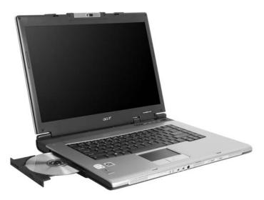
Insert a clip to the emergency eject hole to eject the optical drive tray when the computer is off.
