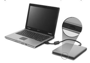
When the power is off, you can eject the drive tray using the emergency eject hole.
