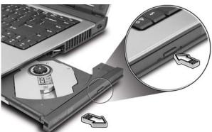
When the power is off, you can eject the drive tray by using the emergency eject hole.
