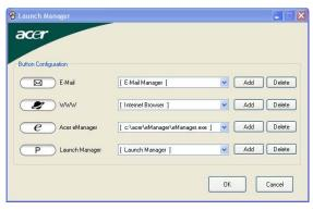
Launch Manager allows you to set the four Easy-launch buttons located above the keyboard. **"Easy-launch buttons" on page 11** for the location of the Easy-launch buttons.
