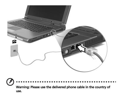
Your computer has built-in Ethernet/Fast Ethernet capabilities. To use the network feature, connect an Ethernet cable from the network jack to an network jack or hub. Consult your network administrator for details.
