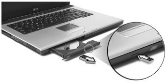
When the power is off, you can eject the drive tray using the emergency eject hole. See page 54.
