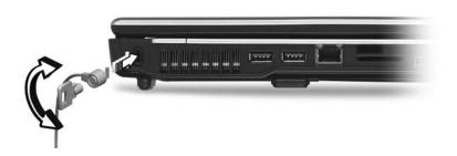
Wrap the computer security lock cable around an immovable object such as a table or handle of a locked drawer. Insert the lock into the notch and turn the key to secure the lock. Some keyless models are also available.
