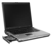
When the power is off, you can eject the drive tray using the mechanical eject hole.
