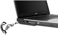
Wrap a computer security lock cable around an immovable object such as a table or handle of a locked drawer. Insert the lock into the notch and turn the key to secure the lock. Some keyless models are also available. The computer comes with 16-bit high-fidelity AC'97 stereo audio, and dual stereo speakers.
