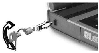
Wrap the computer security lock cable around an immovable object such as a table or handle of a locked drawer. Insert the lock into the notch and turn the key to secure the lock. Keyless models are also available.
