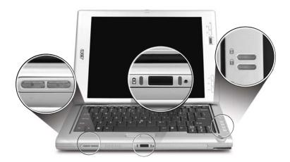
The battery, media, Bluetooth and wireless communication status indicators are visible even when the LCD display is closed.
