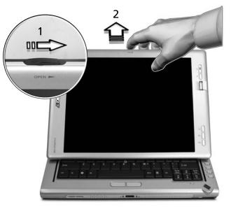
2) Gently pull the display unit from the bottom until it locks into the upright position and use the keyboard to enter data.
