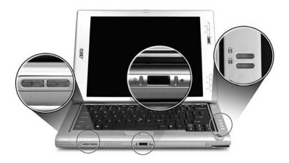
The battery, media, Bluetooth and wireless communication status indicators are visible even when the LCD display is closed.
