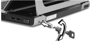
Wrap the computer security lock cable around an immovable object such as a table or handle of a locked drawer. Insert the lock into the notch and turn the key to secure the lock. Keyless models are also available.
