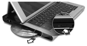
Insert a paper clip to the emergency eject hole to eject the optical drive tray when the computer is off.
