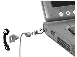
Wrap the computer security lock cable around an immovable object such as a table or handle of a locked drawer. Insert the lock into the notch and turn the key to secure the lock. Some keyless models are also available.
