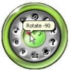
• The right arrow (3 o'clock position) rotates the display output 90 degrees clockwise. This changes the output from landscape to portrait or vice versa. Press the icon as shown.
