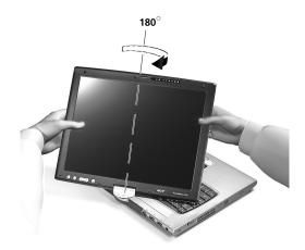
3 With the screen facing away from the keyboard, close the display cover and slide the lock lever to properly secure the screen.
