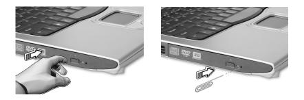
When the power is off, you can eject the drive tray by using the emergency eject hole.
