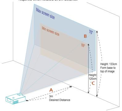
Figure: Fixed distance with different zoom and screen size. (only for X1160Z/ZC/PZ/PZC, X1260/Z/ZC/P/PZ/PZC/K/KC series, X1160/P series is Fixed zoom lens)
