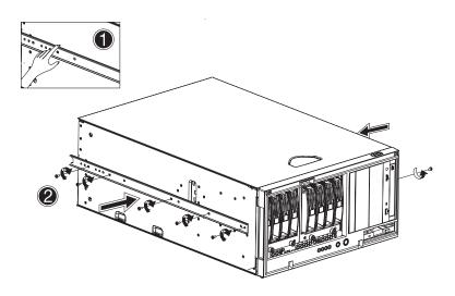
6 Attach the two side handles to the server using four hex head screws for each handle.
