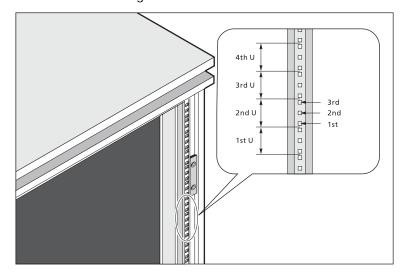
The system occupies 5U in the rack. Count the U positions and hole numbers from the bottom up.
