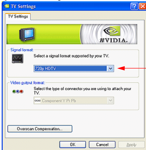
Figure 6.5 TV Settings — HDTV over DVI Connection
