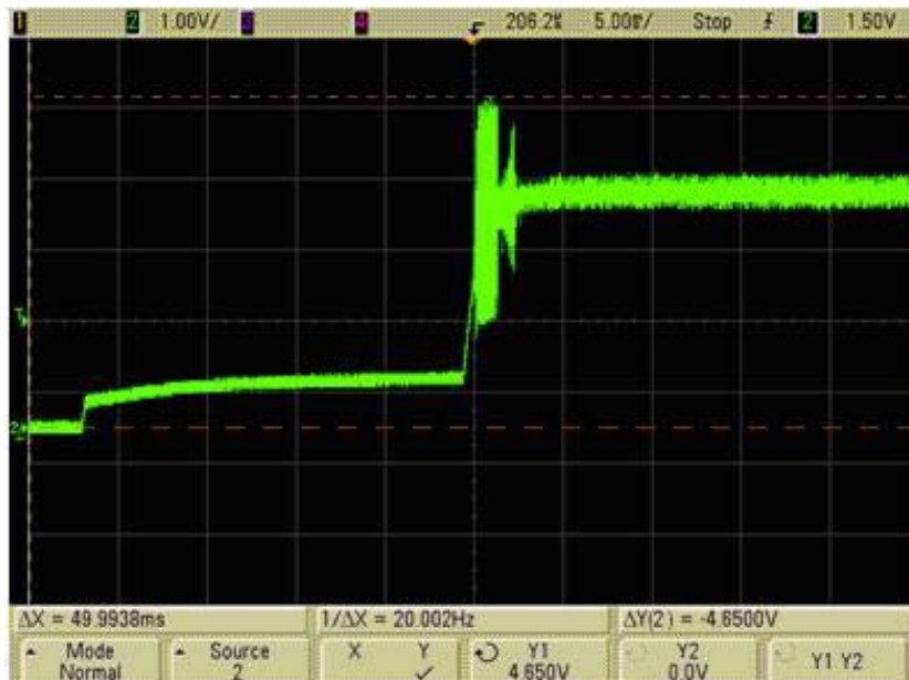
Figure 12. Input Voltage Overshoot >4V (Bad)
