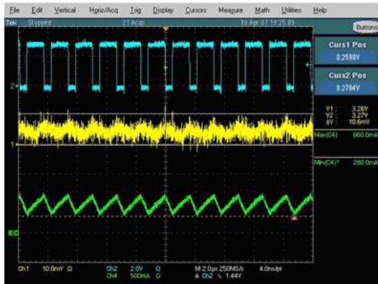
Figure 13. Ceramic 22 \mu F 1210 (X5R) (Good)
