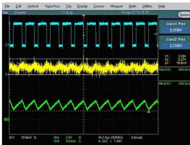
Figure 20. Ceramic 22 \mu F 1210(X5R) (Good)
