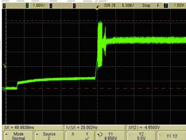
Figure 19. Input Voltage Overshoot >4V (Bad)
