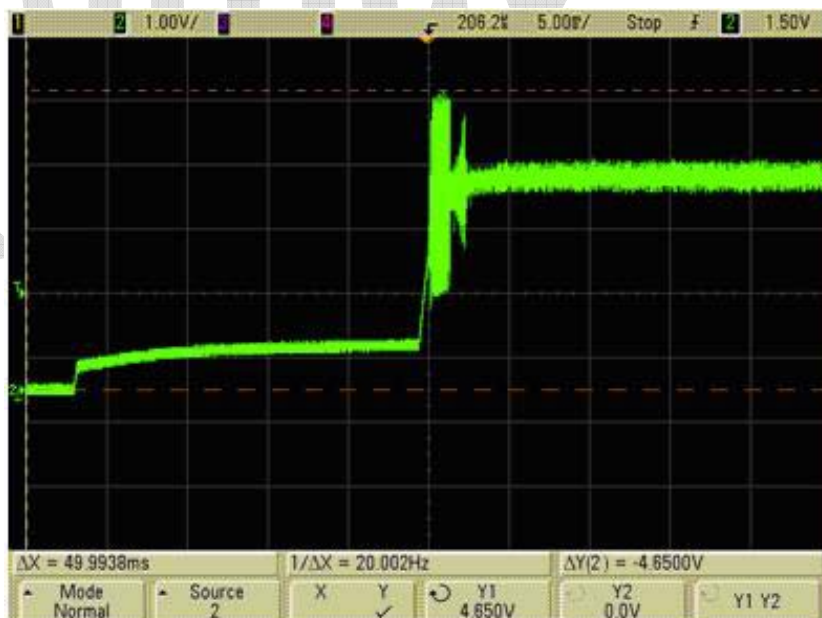
Figure 9. Input Voltage Overshoot >4V (Bad)
