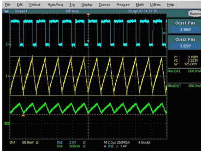
Figure 12. Electrolytic 100 \mu F (Ripple Too High)
