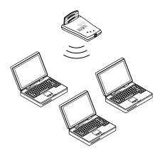
For more complex requirements, you can configure several access points as separate networks at the same site. The access points use different network identifiers called *wireless LAN service areas* (*WLAN service areas*, also called *Extended Service Set Identities* or *ESSID*). Clients can roam within the coverage areas of access points that have the same WLAN service areas. They cannot roam to the coverage areas of access points that are configured with different WLAN service areas.
