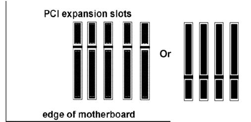
Insert the MegaRAID Express 500 card in a PCI slot as shown below:
