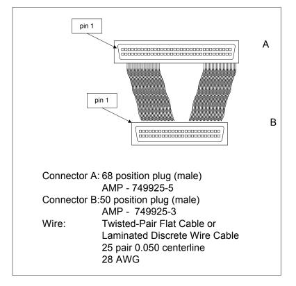
Converting Internal Wide to Internal Non-Wide (Type 30) The cable assembly for connecting internal wide SCSI devices to internal non-wide SCSI devices is shown below:
