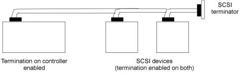
Setup using one connector for one channel
