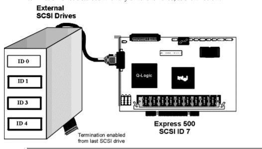
**Terminating Internal and External Disk Arrays** You can use both internal and external drives with MegaRAID Express 500. You still must make sure that the proper SCSI termination and termination power is preserved, as shown below:
