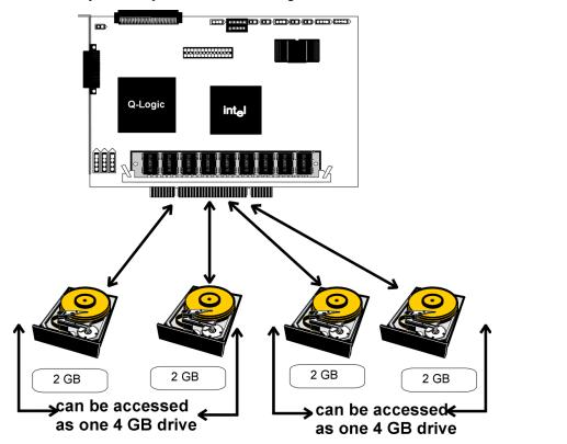
Spanning for RAID 10, RAID 30, or RAID 50
