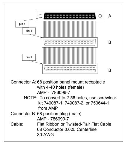
**Connecting Internal and External Wide Devices** The cable assembly for connecting internal wide and external wide SCSI devices is shown below:
