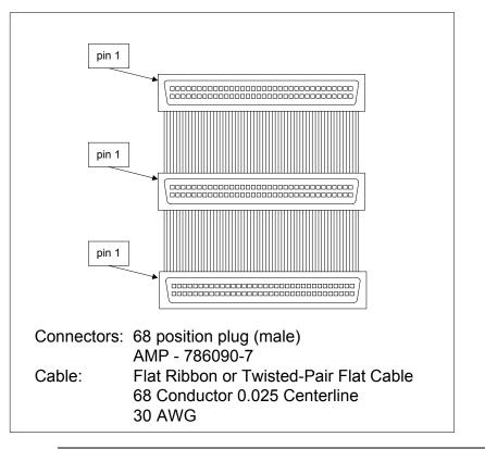
Cable Assembly for Internal Wide SCSI Devices The cable assembly for connecting internal wide SCSI devices is shown below:
