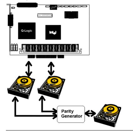
Disk striping writes data across multiple disk drives instead of just one disk drive. Disk striping involves partitioning each drive storage space into stripes that can vary in size from 2 KB to 128 KB. These stripes are interleaved in a repeated sequential manner. The combined storage space is composed of stripes from each drive. MegaRAID Express 500 supports stripe sizes of 2 KB, 4 KB, 8 KB, 16 KB, 32 KB, 64 KB, or 128 KB.
