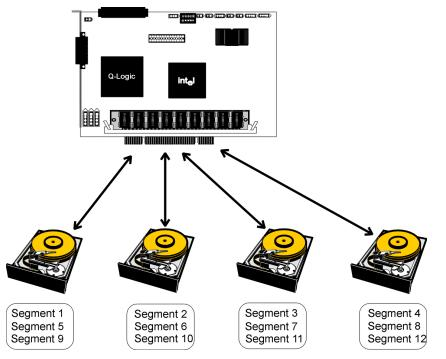
**Stripe Width** Stripe width is a measure of the number of disks involved in an array where striping is implemented. For example, a four-disk array with disk striping has a stripe width of four.
