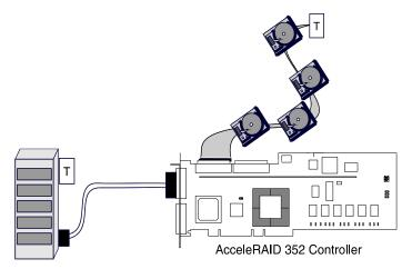
Figure 2-9. Connecting Disk Drives to the AcceleRAID 352
