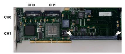
Figure 2-1. AcceleRAID 352 Controller with Connectors
