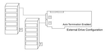
Figure 2-11. Termination with External Drive Configuration
