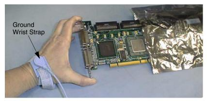
Figure 2-7. Remove the controller from the Anti-static Bag
