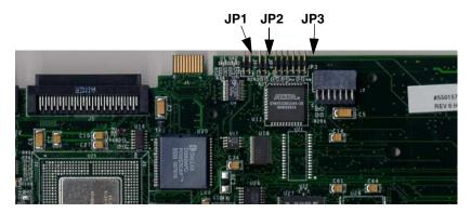
Figure 2-2. AcceleRAID 352 Default Jumper Identification
