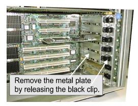
Figure 2-6. Remove the Metal Plate
