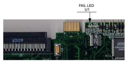
Figure 2-3. AcceleRAID 352 Controller with LED (front)
