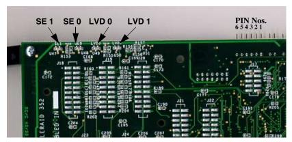
Figure 2-4. AcceleRAID 352 Controller with LEDs and Pin Numbers (back)
