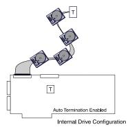
Figure 2-10. Termination with Internal Drive Configuration
