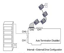
Figure 2-12. Termination with Internal and External Drive Configuration
