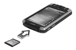
Push the card into the slot using your finger until you feel the card lock and hear an audible system sound. This indicates that the card is properly seated within the slot.
