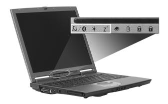
The Wireless, Power and Sleep status indicators (marked area) are visible even when the display is closed.
