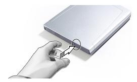
When the power is off, you can eject the drive tray using the emergency eject hole. See page 52.
