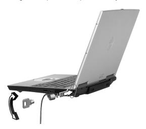
Wrap a computer security lock cable around an immovable object such as a table or locked drawer handle. Insert the lock into the notch and turn the key to secure the lock. Some keyless models are also available.
