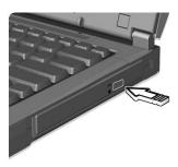
When the power is off, you can eject the drive tray using the emergency eject hole. See page 60.
