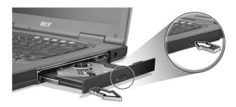
When the power is off, you can eject the drive tray using the emergency eject hole. See page 60.
