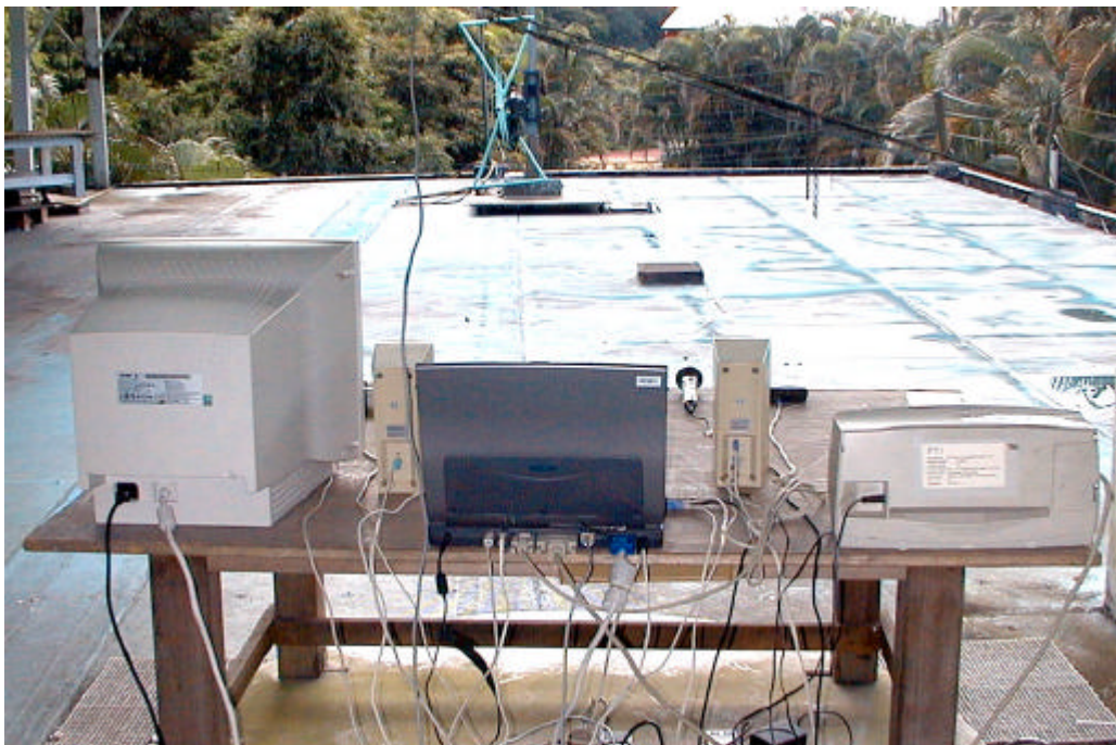
Back View of Highest Radiated Emission Test.
