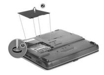
3 Insert the memory module diagonally in the slot (1), and then press down gently until it clicks in place (2).
