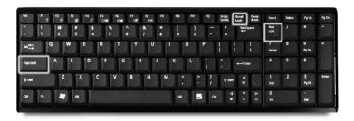
The computer features three lock keys, each with its own status indicator light.
