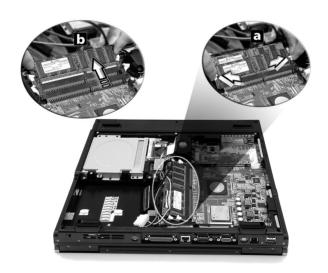
The computer automatically detects the new module and reconfigures the memory.
