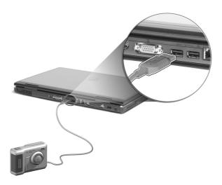
USB is plug and play, which means that you can connect and start using a USB device without having to restart your computer. You can also disconnect the device at any time.
