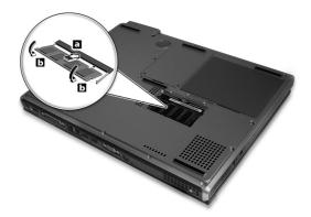
4 Replace the memory compartment cover, and fasten the screw. The system automatically detects the new module and reconfigures the system memory.
