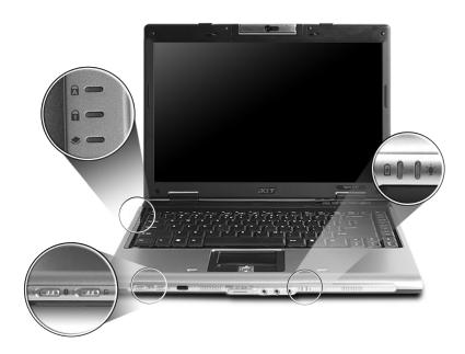
The power, battery, Bluetooth and wireless communication status indicators are visible even when the LCD display is closed.
