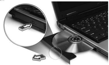
Ilnsert a clip to the emergency eject hole to eject the optical drive tray when the computer is off.
