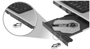
When the power is off, you can eject the drive tray using the emergency eject hole.
