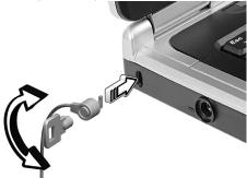
Wrap a computer security lock cable around an immovable object such as a table or handle of a locked drawer. Insert the lock into the notch and turn the key to secure the lock. Some keyless models are also available.
