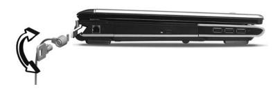
Wrap the computer security lock cable around an immovable object such as a table or handle of a locked drawer. Insert the lock into the notch and turn the key to secure the lock. Some keyless models are also available.
