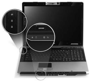
The power, battery and wireless communication status indicators are visible even when the LCD display is closed.
