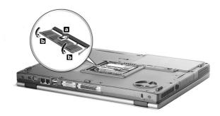
4 Replace the memory compartment door, and fasten the screw.
