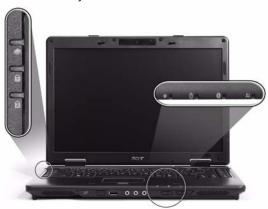
The front panel indicators are visible even when the computer cover is closed up.
