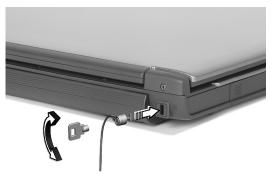
Wrap the computer security lock cable around an immovable object such as a table or handle of a locked drawer. Insert the lock into the notch and turn the key to secure the lock. Some keyless models are also available.
