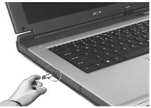
When the power is off, you can eject the drive tray by using the emergency eject hole.
