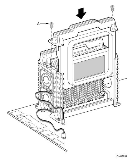
Figure 11. Install the Termination Card
