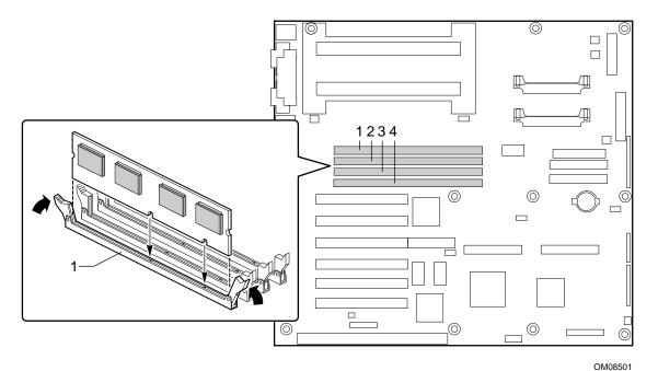
Figure 12. Installing DIMMs
