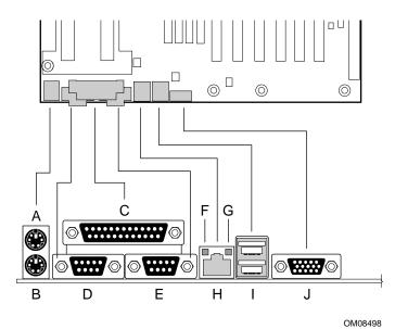
**Figure 1. Back Panel Connectors**
