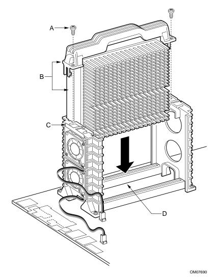
Figure 9. Install Processor
