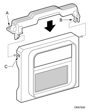
Figure 10. Attaching the Retention Mechansim to the Termination Card
