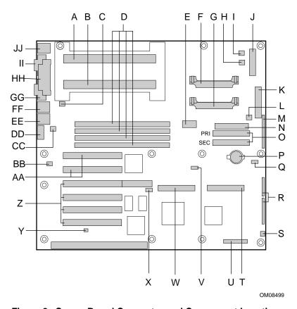
Figure 2. Server Board Connector and Component Locations
