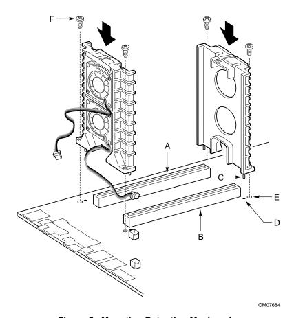
Figure 5. Mounting Retention Mechansim
