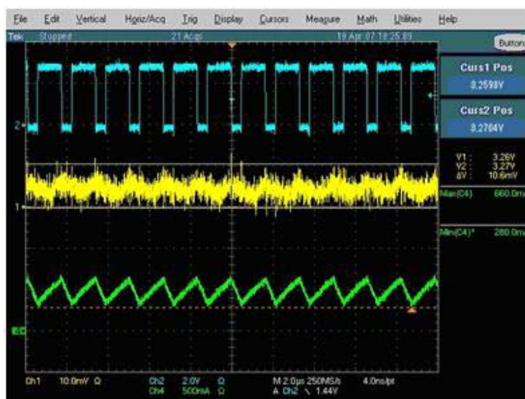
Figure 9. Ceramic 22 \mu F 1210 (X5R) (Good)
